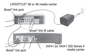
When the connections are completed, you can operate either system using the RC-38S remote.
